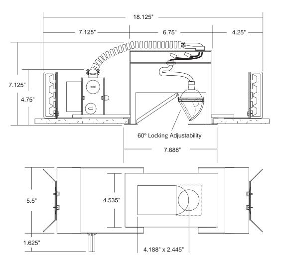
Provided with two (2) 14 gauge steel butterfly type brackets for black iron installations.
